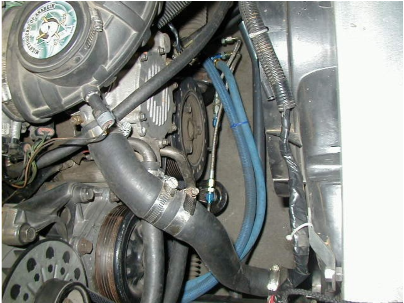
This pictures shows the routing of the lines across in front of the engine.
