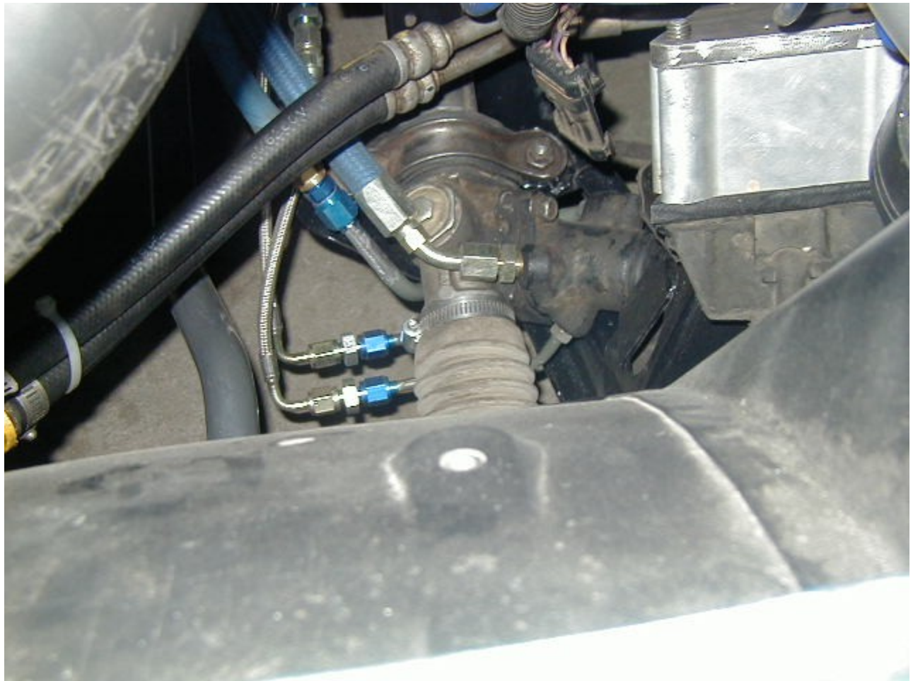
This shows the pressure and return lines at the rack after the install was complete.
