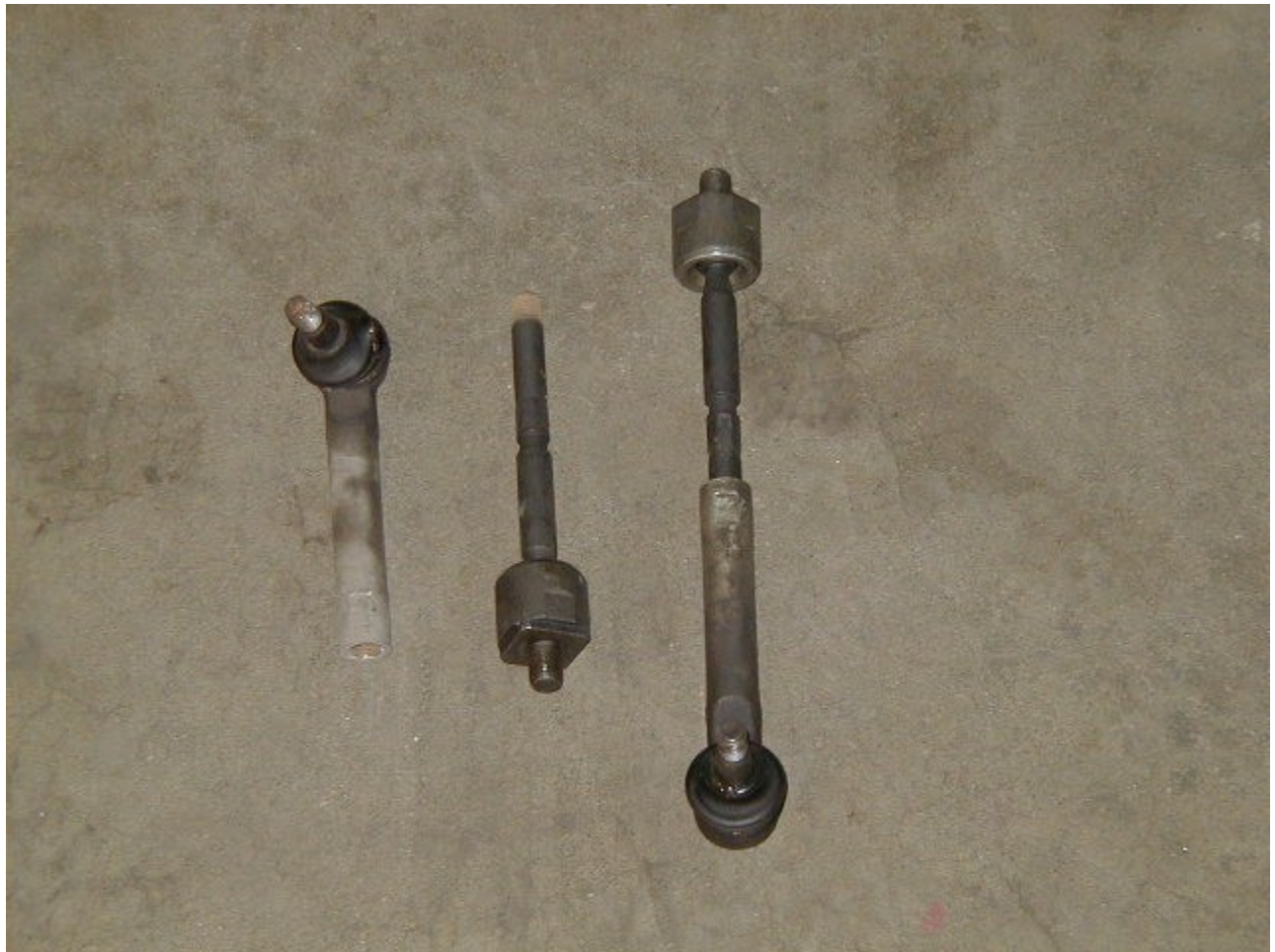
This shows a Celica inner, a Subaru outer and the 2 connected.
