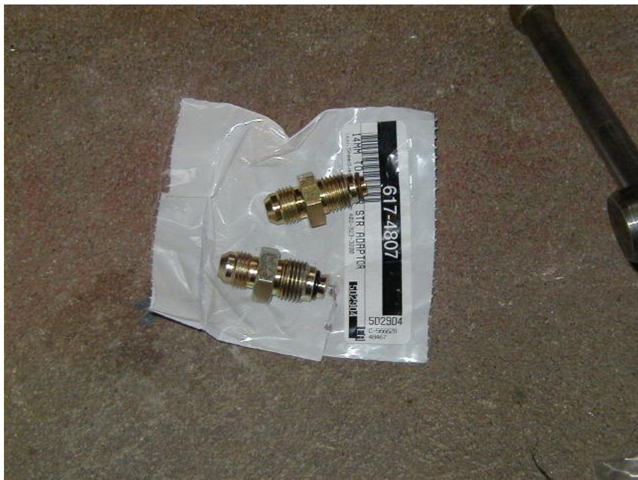
These are power steering adapters I bought from Speedway racing. They thread right into the GM pump and the pressure side of the Forrester rack.
